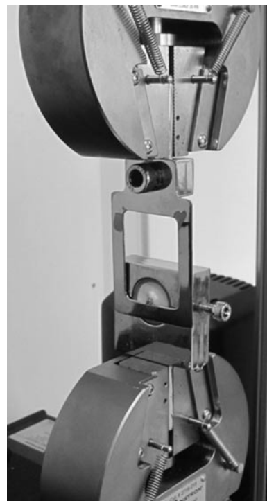
Figure 1 De-bonding plate, mounting jig and tooth with bracket
